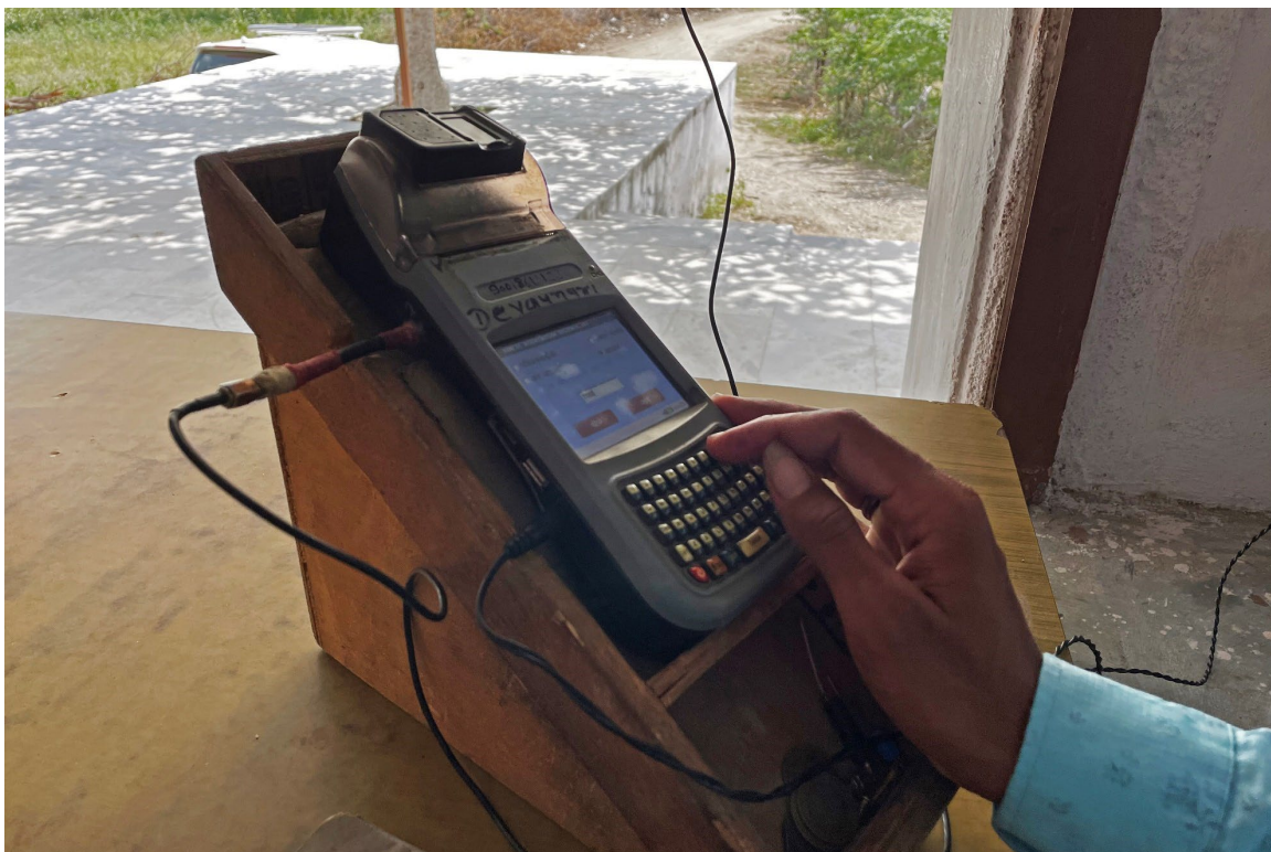
A ration shop dealer in a village in Rajasthan with the machine used for Aadhaar-based biometric authentication. The machine requires internet access to authenticate biometric IDs before people can get the subsidized or free food grains to which they are entitled each month, September 2022. © 2022 Jayshree Bajoria/Human Rights Watch
